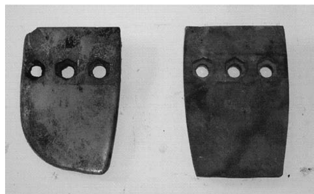
Figure 1. Illustration of used and new mixer blade
